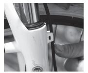
**6** - If your frame allows , route all hoses, correctly fastening them against the frame. Make sure that the hoses do not impede the steering and are not kinked.
