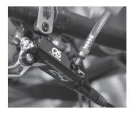
**6** - Remove the fill syringe from the calliper. Securely fasten the bleed nipple back into position. Wipe up any fluid that has spilled from the calliper.
