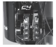
**5** - Check that the calliper is aligned in relation to the rotor and that the rotor is central between the pads. If not adjust accordingly by adjusting the calliper fixing bolts. The rotor should not 'scuff' against the pads.
