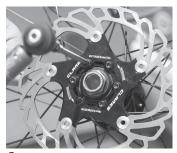
**2** - Fit the rotors to the front and rear wheels using the 6 x T25 Tork head bolts supplied. Finger tighten all bolts, then torque up all bolts, tightening opposite bolts going around the rotor to avoid distortion. Fix the wheels back into the frame.
