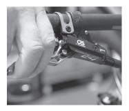
7 - Test your brakes. If all the air has been cleared from the system, the lever should feel 'firm' and 'responsive'.
