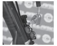
**3** - Gradually depress the syringe at the calliper, pushing the fluid from the calliper through to the lever syringe.
