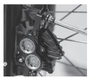
**3** - Remove the calliper pad spacer and fix the callipers to the mounting points on the front and rear forks. If required - fasten the I.S. bracket (or Post Mount bracket) to the bike fork mounting points using 2 x M6 x 18mm bolts supplied, and then fix the calliper to the bracket. Do not tighten the calliper bolts at this stage.
