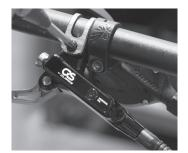
1 - Fit the front and rear lever assemblies to the handlebar. Tighten the lever clamp bolts using a T25 Torx driver. Recommended torque setting - 6-8NM
