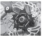
${\bf 2}$  - Fit the rotors to the front and rear wheels using the 6 x T25 Torx head bolts supplied. Finger tighten all bolts, then torque up all bolts, tightening opposite bolts going around the rotor to avoid distortion. Fix the wheels back into the frame.
