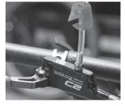
**4** - Continue this process until no air bubbles can be seen exiting the system into the drain syringe.
