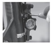
**1** - Remove the calliper bleed bolt and attach the syringe (fill). Finger tighten the syringe only.
