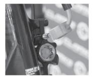
**3** - Gradually depress the syringe at the calliper, pushing the fluid from the calliper through to the lever syringe.
