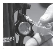
**5** - Remove the drain syringe from the lever. Securely fasten the bleed nipple back into position. Wipe up any fluid that has spilled from the lever.
