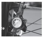
$\boldsymbol{3}$  - Remove the calliper pad spacer and fix the callipers to the mounting points on the front and rear forks. If required - fasten the I.S. bracket (or Post Mount bracket) to the bike fork mounting points using 2 x M6 x 18mm bolts supplied, and then fix the calliper to the bracket. Do not tighten the calliper bolts at this stage.
