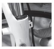
6 - If your frame allows, route all hoses, correctly fastening them against the frame. Make sure that the hoses do not impede the steering and are not kinked. Always test your brakes for effectiveness before riding your bike.
