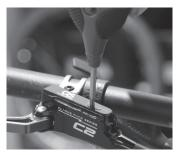
**2** - Remove the lever bleed bolt and attach the syringe (drain). Finger tighten the syringe only.
