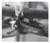
**1** - Fit the front and rear lever assemblies to the handlebar. Tighten the lever clamp bolts using a T25 Torx driver. Recommended torque setting - 6-8NM
