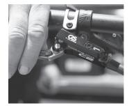
**7** - Test your brakes. If all the air has been cleared from the system, the lever should feel 'firm' and 'responsive'.
