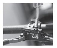
**6** - Remove the fill syringe from the calliper. Securely fasten the bleed nipple back into position. Wipe up any fluid that has spilled from the calliper.
