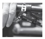
4 - With the calliper in place over the rotor, apply pressure to the lever. This will help to centralise the callipers over the rotor. With the brake lever still applied tighten the calliper bolts to the Post Mount or I.S. fixings.
