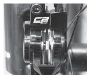
**5** - Check that the calliper is aligned in relation to the rotor and that the rotor is central between the pads. If not adjust accordingly by adjusting the calliper fixing bolts. The rotor should not 'scuff' against the pads.
