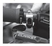
1 - Fit the front and rear lever assemblies to the handlebar. Tighten the lever clamp bolts using a 5mm allen key.
