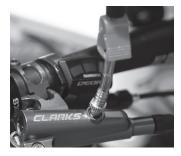
**2** - Attach the syringe (drain) to the lever bleed point.
