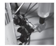
4 - Gradually depress the syringe at the calliper, pushing the fluid from the calliper through to the lever syringe.
