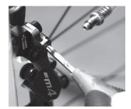
**3** - Remove the bleed nipple from the calliper and attach the syringe (fill).
