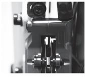
**5** - Check that the calliper is aligned in relation to the rotor and that the rotor is central between the pads. If not adjust accordingly.
