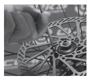
2 - Fit the rotors to the front a rear wheels using the 6 x T25 Torx head bolts supplied. Tighten opposite bolts going around the rotor to avoid distortion. And fix the wheels back into the frame.
