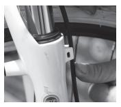
**6** - Route all hoses, correctly fastening them against the frame. Make sure that the hoses do not impede the steering and are not kinked.
