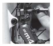
**3** - Remove the calliper pad spacer and fix the callipers to the mounting points on the front a rear forks. If required - fasten the I.S. bracket (or Post Mount bracket) to the bike fork mounting points using 2 x M6 x 18mm bolts supplied, and then fix the calliper to the bracket. Do not tighten the calliper bolts at this stage
