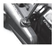
1 - To begin the bleed process remove the bleed nipple from the lever assembly.
