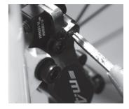
7 - Remove the fill syringe from the calliper. Securely fasten the bleed nipple back into position.
