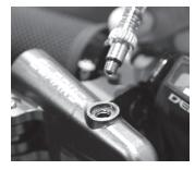
6 - Remove the drain syringe from the lever. Securely fasten the bleed nipple back into position.
