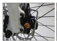
With the brake lever still applied finish fastening the calliper to I.S Bracket / Bike.
