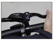
Apply Pressure to the lever this will help to centralize the calliper to rotor.
