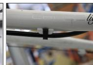
Ensure the hose is correctly fastened to the bike frame / Fork.
