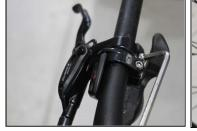
To begin the assembly Fit the lever to the handlebar, tighten the 5mm Allen bolt located on lever clamp.
