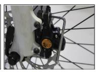
Fasten the I.S Bracket to bike using the 2 M6\*18MM Bolts provided, If P.M mounting skip to next step.
