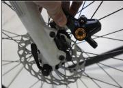
Fasten rotor to wheel using the 6 x t25 Torx head bolts supplied.
