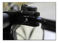
Turn the reach adjustment located on the inside lever blade clockwise to increase distance from handle bar or anti clockwise to decrease the distance from handlebar.
